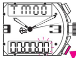
The days (max. 99 days) on the upper display flash and pressing pushpiece B briefly makes the H, MIN and SEC on the lower display flash in turn.
