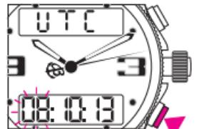
Press pushpiece B briefly: the H and MIN on the display flash in turn.
