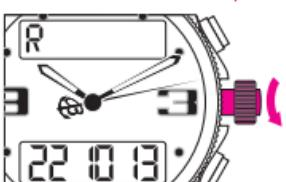
The respective synchronization of analog H, MIN and SEC (hands) is done by rotating the crown. N.B. The SEC only move clockwise.
