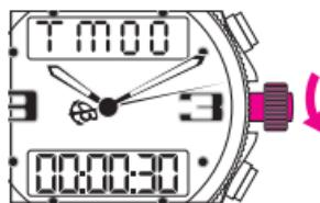
The respective adjustments of the days, H, MIN and SEC is done by rotating the crown. Push the crown back to position 1.
