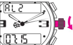
The respective adjustments of H and MIN on the alarm are done by rotating the crown. Push the crown back to position 1.
