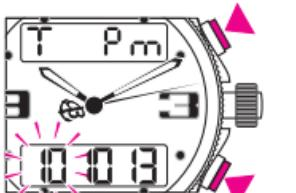
The time may be displayed in 24H or AM/PM mode by briefly pressing pushpiece A. In AM/PM mode, the upper display may be suppressed by pressing A.
