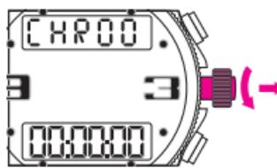
If the seconds hand is not precisely positioned at 12 o'clock in **CHR** mode, pull the crown out to position 2 and turn forwards to reposition the hand at 12 o'clock. Push the crown back in to position 1.
