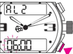
Press pushpiece B briefly: the H, MIN displays flash in turn.
