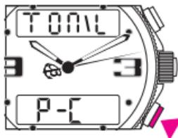
**P-C** appears in lower display: audible confirmation signal each time pushpieces are pressed + hour pips for time being measured.
