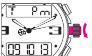
Press pushpiece B briefly: the hours, minutes and seconds (H, MIN and SEC) of the display flash in turn.
