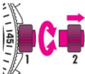
Crown: backlighting of display by pressing, selection of functions by rotation (position 1); functions setting or choice of language by rotation (position 2).
