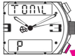
P appears in lower display: audible confirmation signal each time pushpieces are pressed.
