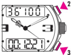
Chronograph stopped: upper display indicates the measurement to the nearest 1/100th of a second and alternatively (ADD), the number of days elapsed.
