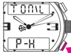
P-H appears in lower display: audible confirmation each time pushpieces are pressed + hour pips.
