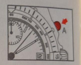
2. To interrupt the time measurement process, press pushpiece A again. To resume time measurement, press pushpiece A. A number of separate time spans can thus be measured cumulatively.
