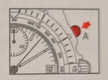
2. To stop the chronograph, press pushpiece A again. Elapsed time is measured in hours (totalizer 1), minutes (totalizer 2) and 1/5ths of a second (hand C).
